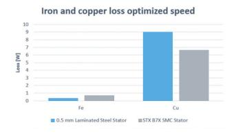
If we look at the figure above, it is evident that the iron loss will be slightly higher for SMC compared to laminated iron, but the copper loss is significantly lower when using the optimized SMC shape.
