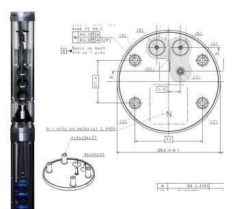
Subsequently, the four towers were machined from solid rod as shown in the figure below, including processing of internal threads. The four towers were mounted on the plate and then attached with a resistance welding.
