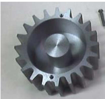
Figure 4 SMC pot core designed with external cooling ribs v
